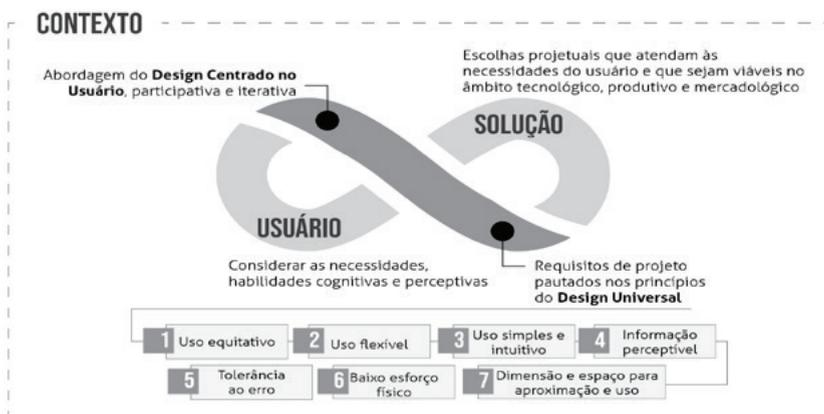
Figura 1. Relação entre conceitos para o desenvolvimento de produtos acessíveis. Fonte: As autoras (2021), baseado em: Connell et al. (2001), Clarkson; Coleman (2015) nor a separate specialism, but as a general approach to designing in which designers ensure that their products and services address the needs of the widest possible audience, irrespective of age or ability. Inclusive Design (also known [in Europe] as Design for All and as Universal Design in the USA, Smythe (2018).
