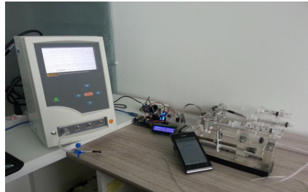
Figure 1: Syringe Infusion Pump Prototype under development. The system is triggered remotely by mobile applications that collect health information systems data tested by IDA 4 Plus Infusion Analyzer at NUTES.
