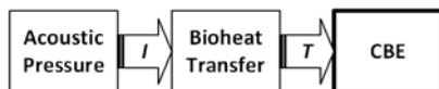
Fig. 3: Coupling between the different modules for therapeutic US heating simulation, where I is the sound wave intensity and T is the system temperature.
