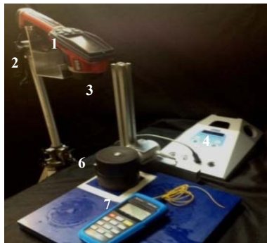
Figure 2: Experimental arrangement for US irradiation in the cylindrical four-layer phantom. In the image: 1) Infrared Camera; 2) Tripod; 3) Support for the US transducer; 4) Therapeutic US Equipment; 5) Transducer UST; 6) Cylindrical Four-layer Phantom and 7) Digital Thermometer.
