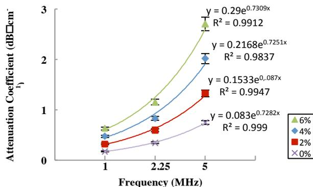
Figure 4: Ultrasound attenuation (dB/cm) with frequency (MHz) of the phantoms progressive reduction in graphite powder concentration @ 26 °C.
