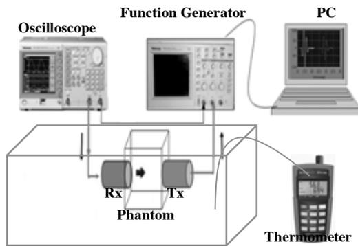
Figure 2: Experimental procedures set-up for characterization of acoustic properties of the phantoms.
