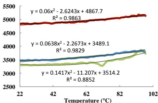
Figure 5: Specific heat (J/kg·K) of the phantoms with temperature (°C) with progressive reductions in graphite powder concentration (-2, -4 and -6 %).
