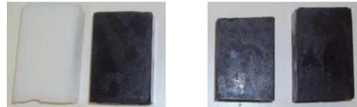
Figure 1: Final aspect of the phantoms with progressive reduction in graphite powder concentration.
