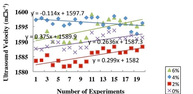
Figure 3: Ultrasound propagation velocity (m□s<sup>-1</sup>) with repeatability in time for the phantoms progressive reduction in graphite powder concentration at 26 °C.
