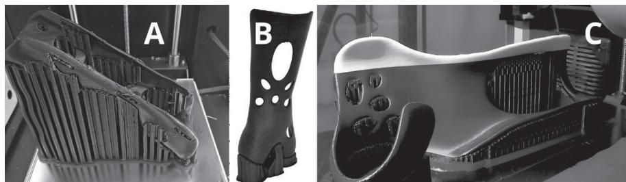
Figure 06 - Angled ABS print on Creality CR200B with extensive supports (A); Support oriented matte-finished PLA-CF prototype (B); ABS orthosis on Creality K1 Max using optimal orientation and high-density support interface (C).
