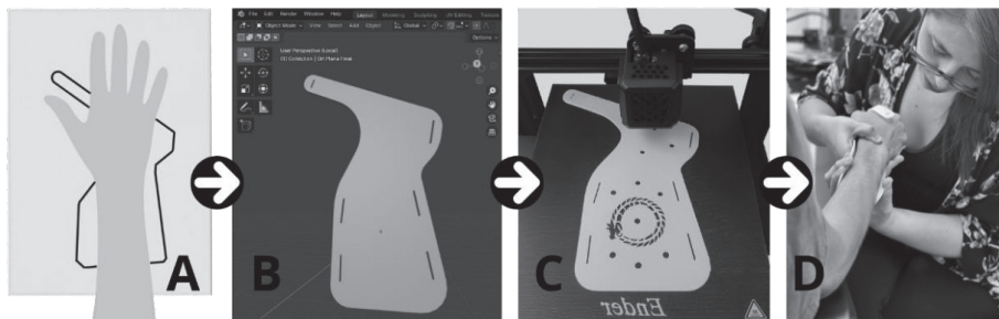
Figure 01 - Paper mold of the orthosis (A); 3D model in Blender (B); Orthosis during printing (C); Orthosis thermoforming (D).
