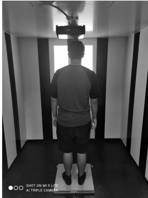
Figure 1. Experimental set-up with an adult standing on the force plate, inside the moving room.
